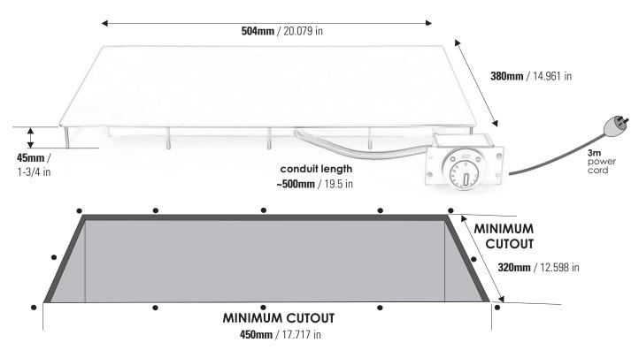
The control box must be firmly fastened to a non-moving surface. Conduit + power cord to be secured. **CAUTION**: Do not snap, pull or twist the conduit during installation.
