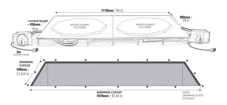
The control box must be firmly fastened to a non-moving surface. Conduit + power cord to be secured. CAUTION: Do not snap, pull or twist the conduit during installation. Warranty becomes void if capillary tube (thermostat) inside the conduit is damaged during installation.
